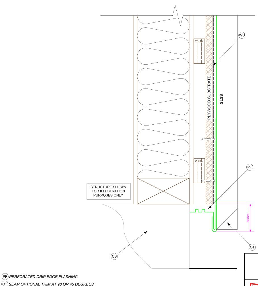
SINGLE LOCK STANDING SEAM (SLSS) **BOTTOM WITH PERFORATED FLASHING**
